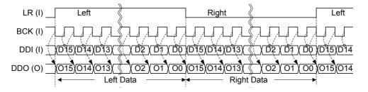
During playback, the 16-bit playback data is input serially from the MSB to the DDI pin in synchronization with the clock signal of the BCK pin. The DDI pin input data is taken in the LSI at the rising edge of the BCK clock signal. The recording data is output from the DDO pin at the falling edge of the BCK clock signal during recording.
