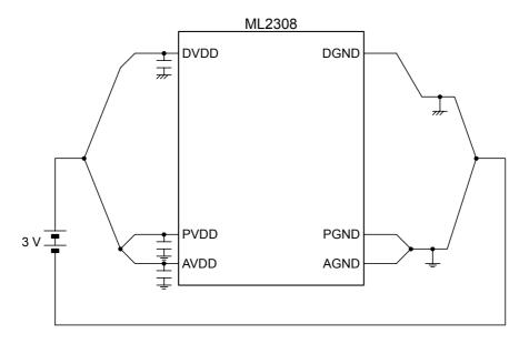
Do not arrange the wiring as shown below.
